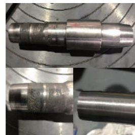
Pump shaft repair
