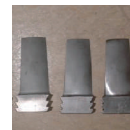
Steam turbine blade repair
