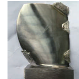
Blade notch repair
