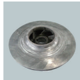
Hastelloy impeller repair
