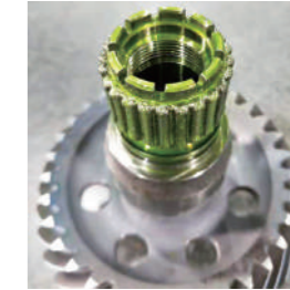
Repair of external spline shaft parts
